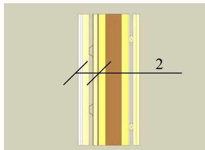
Figure 2: The load bearing exterior wall. The layers indicated with the number 2 is from right to left; 2 layers of 13 mm gypsum board;  $45 \times 45 \text{ mm}^2$  wooden beams and mineral wool; Gyproc resilient acoustic profile (AP); board lamella.
